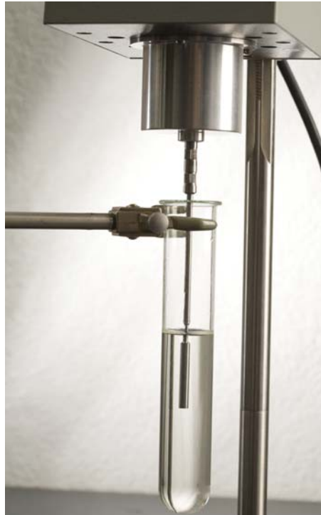
Figure 3.3 Viscometer device used to determine a liquid's absolute or kinematic viscosity.
