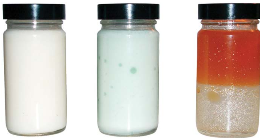
Figure 4.6 AMSOIL Synthetic Compressor Oil (shown far right), separates from water rapidly to inhibit rust formation and preserve wear protection.
