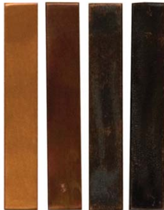
Figure 4.5 Examples of Copper Corrosion test results (left). ASTM Copper Corrosion Standards (above).
