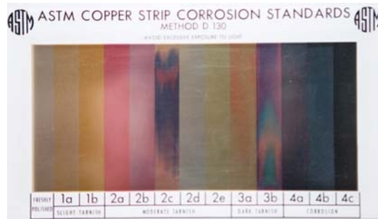
Figure 4.5 Examples of Copper Corrosion test results (left). ASTM Copper Corrosion Standards (above).
