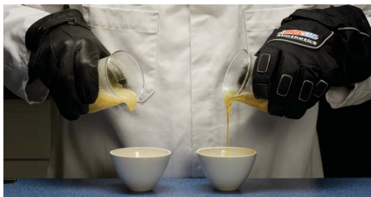
Figure 3.5 A lubricant's pour point is a key measure of its ability to flow at low temperatures.
