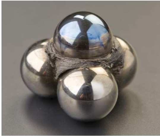
Figure 4.2 Example of welded test balls
