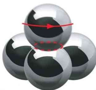
Figure 4.3 The Four-Ball Wear Test assesses the average wear scar diameter to determine a lubricant's ability to reduce wear.
